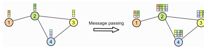
Figure 2. A small example of message-passing within a Graph Neural Network as taken from [5].
